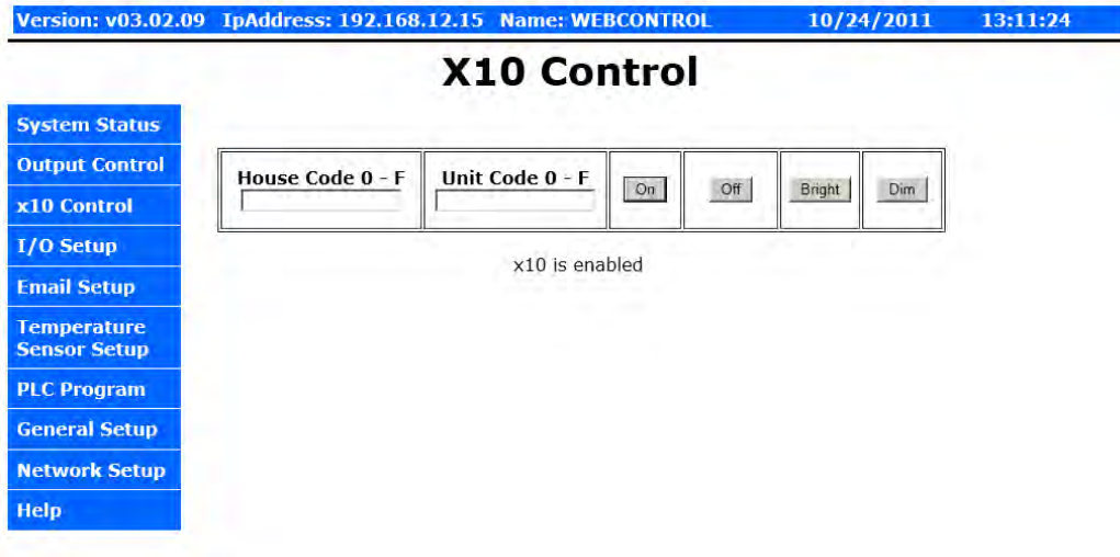
Figure 6.0 WebControl™ X10RF Control
